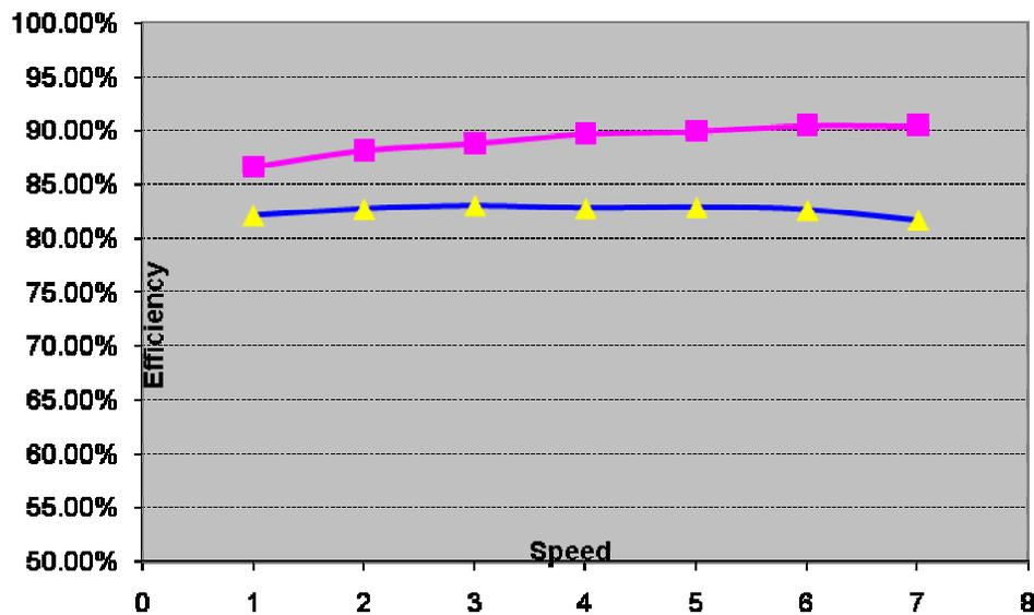
Fig. 3. Efficiency with load resistance of 1.34 and 0.565 ohms
