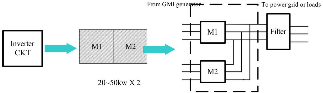
Fig. 3. Inverter based on two modules to double power capability
