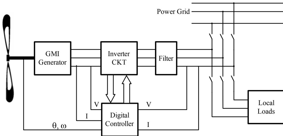
Fig. 1. Overall system description of direct-driven wind turbine generator system
