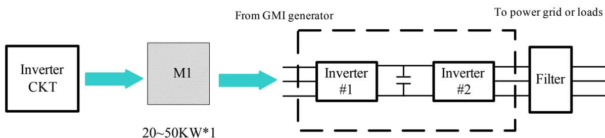
Fig. 2. Basic modular inverter as building-block
