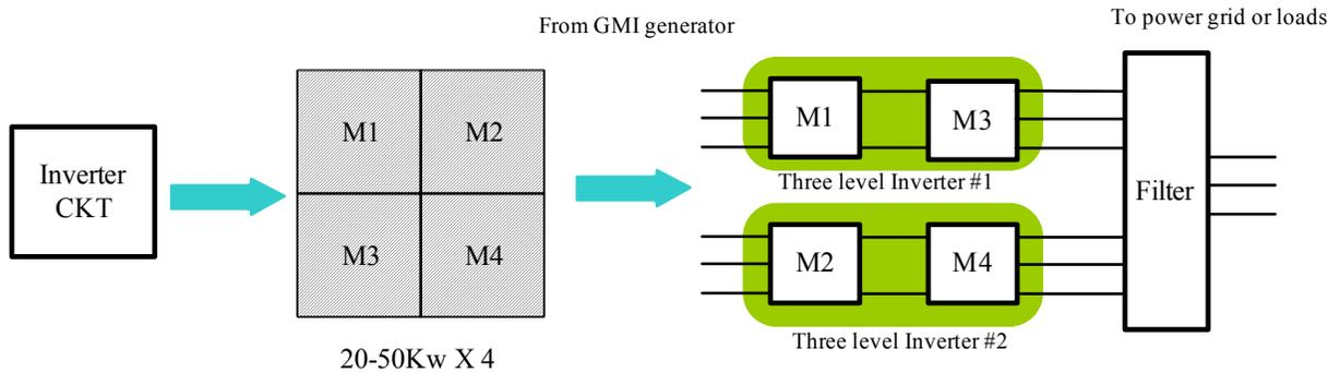
Fig. 4. Two 3-level inverters for much large power capability using 4 modules of building-block
